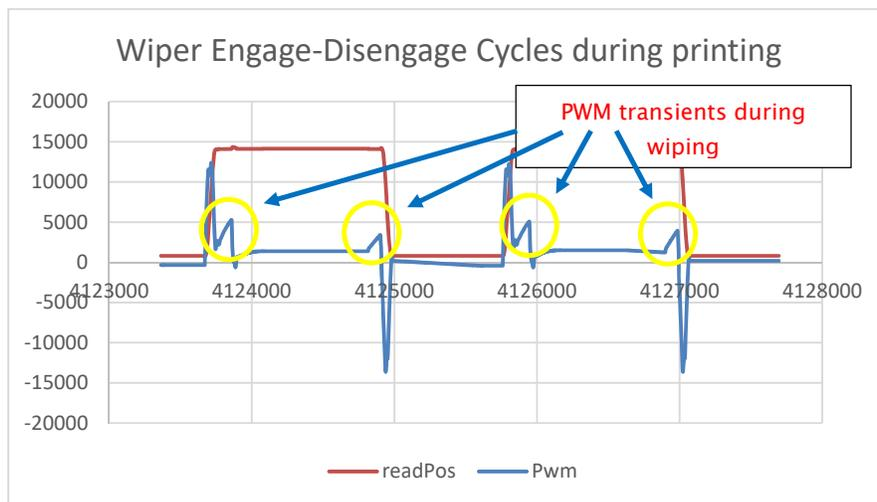
Figure 3: Wiper Engage Motor PWM and Height
