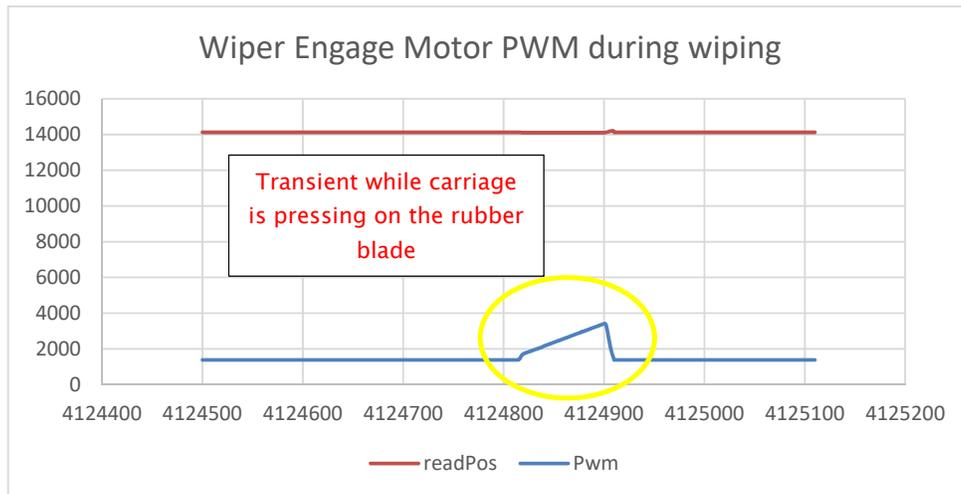
Figure 2: Wiper Engage Motor PWM and Height
