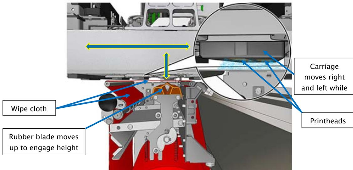
Figure 1: View of wiper and carriage
