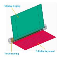
The panel, keyboard and panel back plate is scrolled and collapsed on a rotational internal tube. A torsion spring is attached to the tube with compressed force and locked by a latch. The latch could be in form of ratchet wheel and pawl mechanism. Once the latch is released, the torsion spring makes the tube rotate by spring force and pop out the foldable keyboard and panel.
