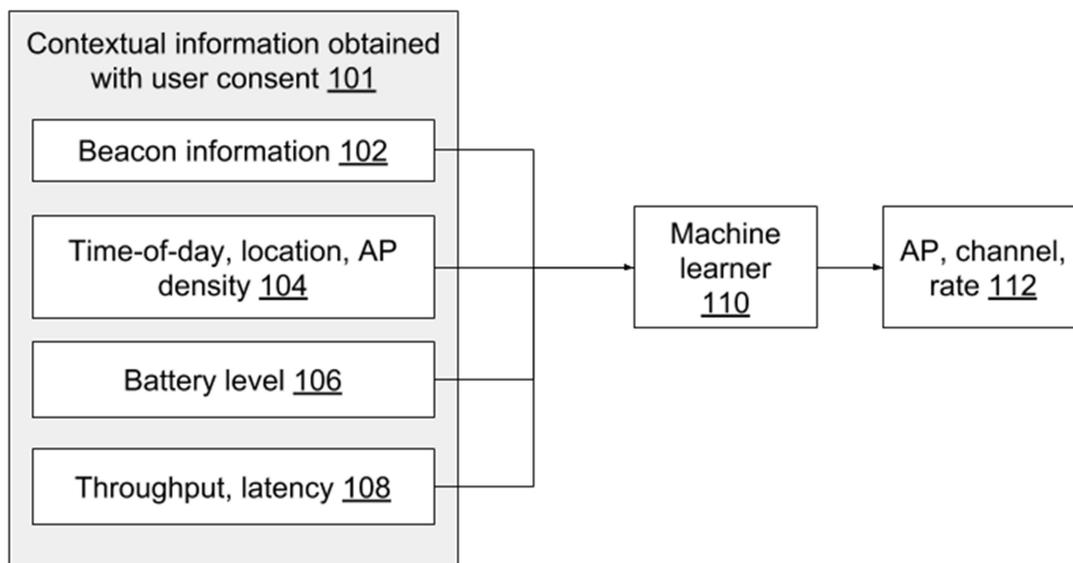
**Fig. 1: Applying machine learning to select Wi-Fi parameters**
