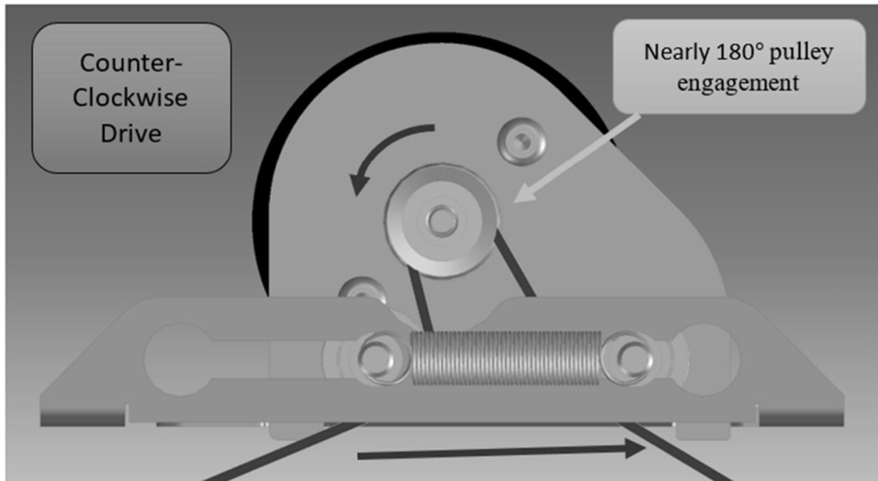
Figure 4 - Belt tensioner with motor driving counter clockwise
