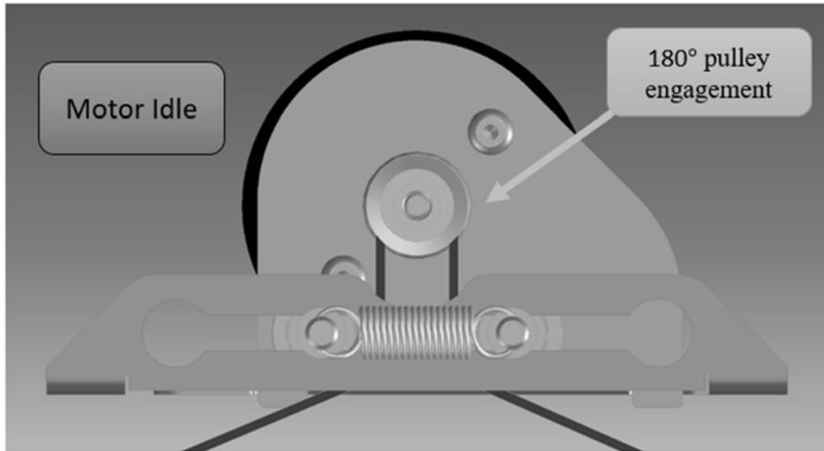
Figure 2 - Belt tensioner with motor idle
