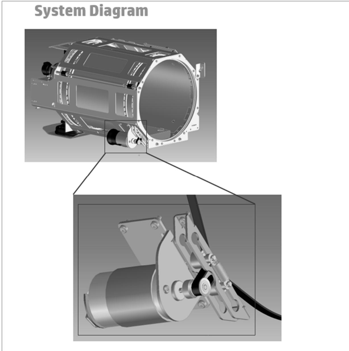
*Figure 1 - System view of belt tensioner*
