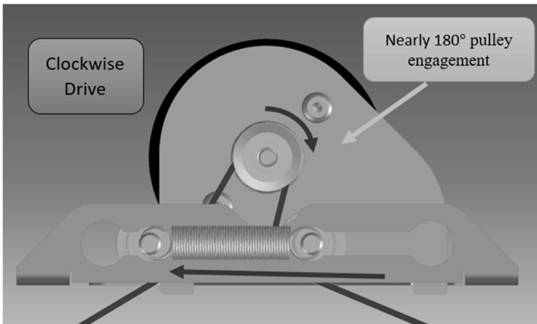
Figure 3 - Belt tensioner with motor driving clockwise
