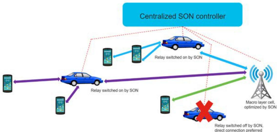
**FIG. 1: A cluster with three relays, where SON switches two on and keeps one off, optimizing the cluster as a whole**
