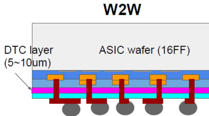
Figure 2A: Example wafer-to-wafer on-die capacitor configuration
