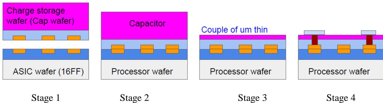
Figure 1: Example fabrication steps of a massive on-die capacitor for ICs
