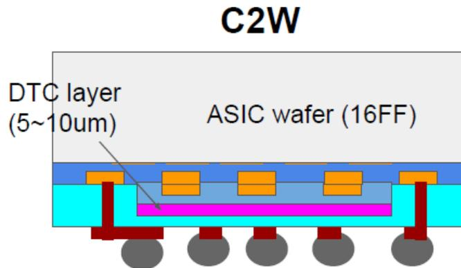
Figure 2B: Example chip-to-wafer on-die capacitor configuration
