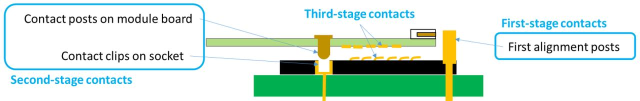
This design allows the large alignment posts for electrical contacts allows a larger surface area for electrical connection and enabling higher current applications. In addition, fewer spring contact required for power allows lower compression force, which in turns places less mechanical strain on the system and module board.
