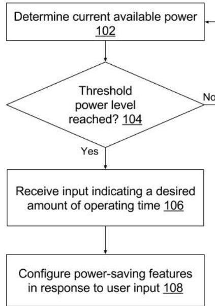
**Fig. 1: Dynamic adjustment of power consumption based on time or event goals**
