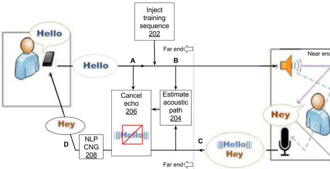
**Fig. 2: Acoustic echo canceler with below-masking-threshold training sequence**
