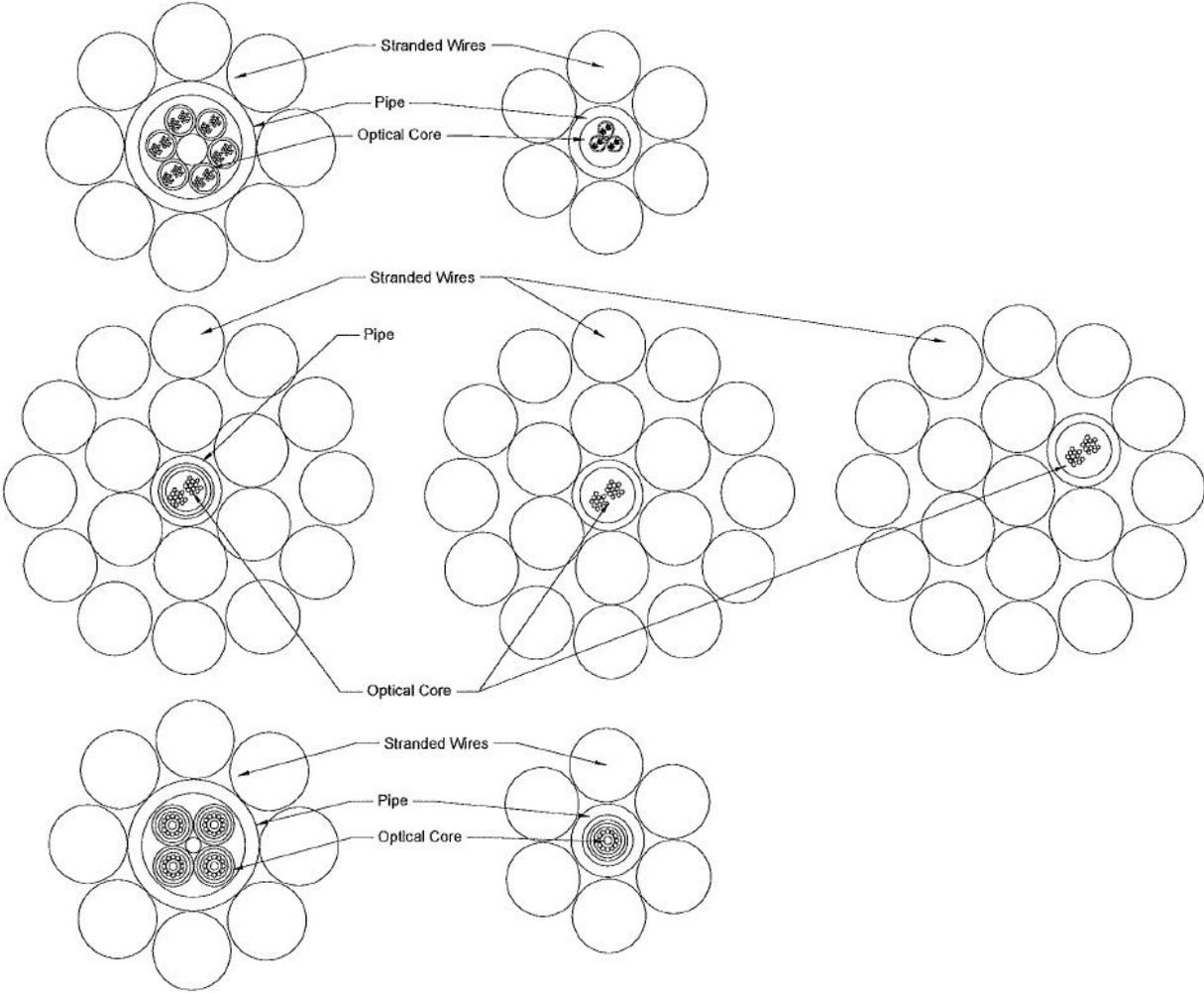
Typical OPGW cable structures which incorporate optical cores as discussed above.
