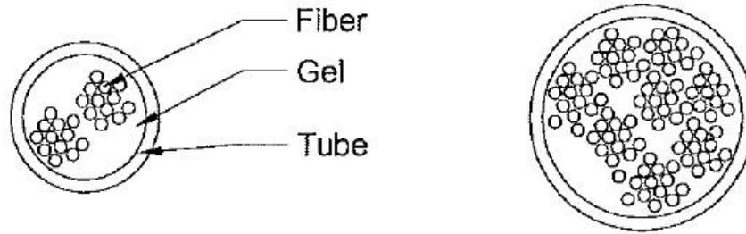
Stainless Steel Tube Optical Ground Wire Core - This core consists of a stainless steel tube that is gel filled or dry blocked and placed inside of an aluminum pipe or aluminum extrusion or used straight or helixed in the cable structure.
