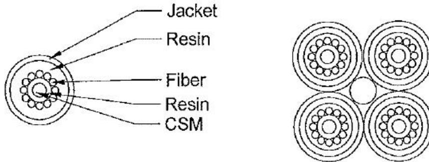
Tight Structure Optical Ground Wire Core - This core consists of one or many tight structure units. A tight structure unit consists of a center member that has fibers helixed around it encased in epoxies and silicones with an overall jacket. This core is typically placed inside of an aluminum pipe or aluminum extrusion in the cable structure.
