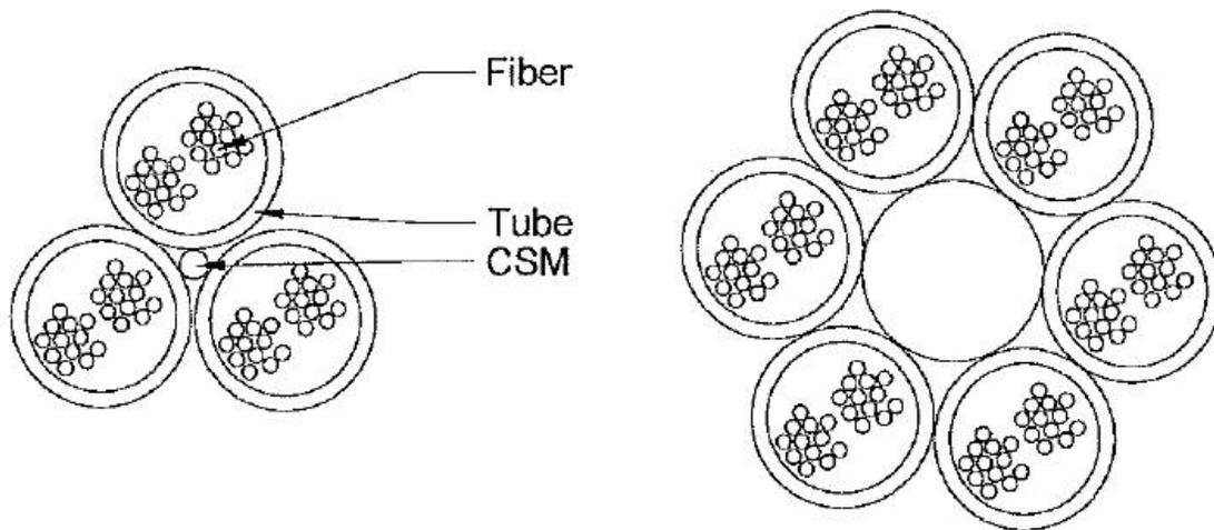
Loose Tube Optical Ground Wire Core (LT-OPGW) - This core typically consists of a central strength member surrounded by helixed tubes that are gel filled or dry blocked and made of plastic. This core is typically placed inside of an aluminum pipe or aluminum extrusion in the cable structure.
