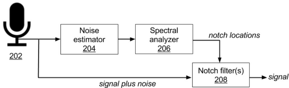
**Fig. 2: Placement of notches in notch filter**
