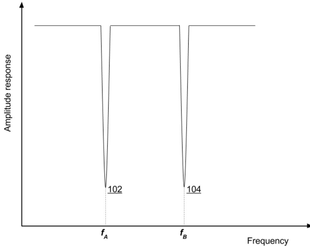
**Fig. 1: Response of a notch filter**
