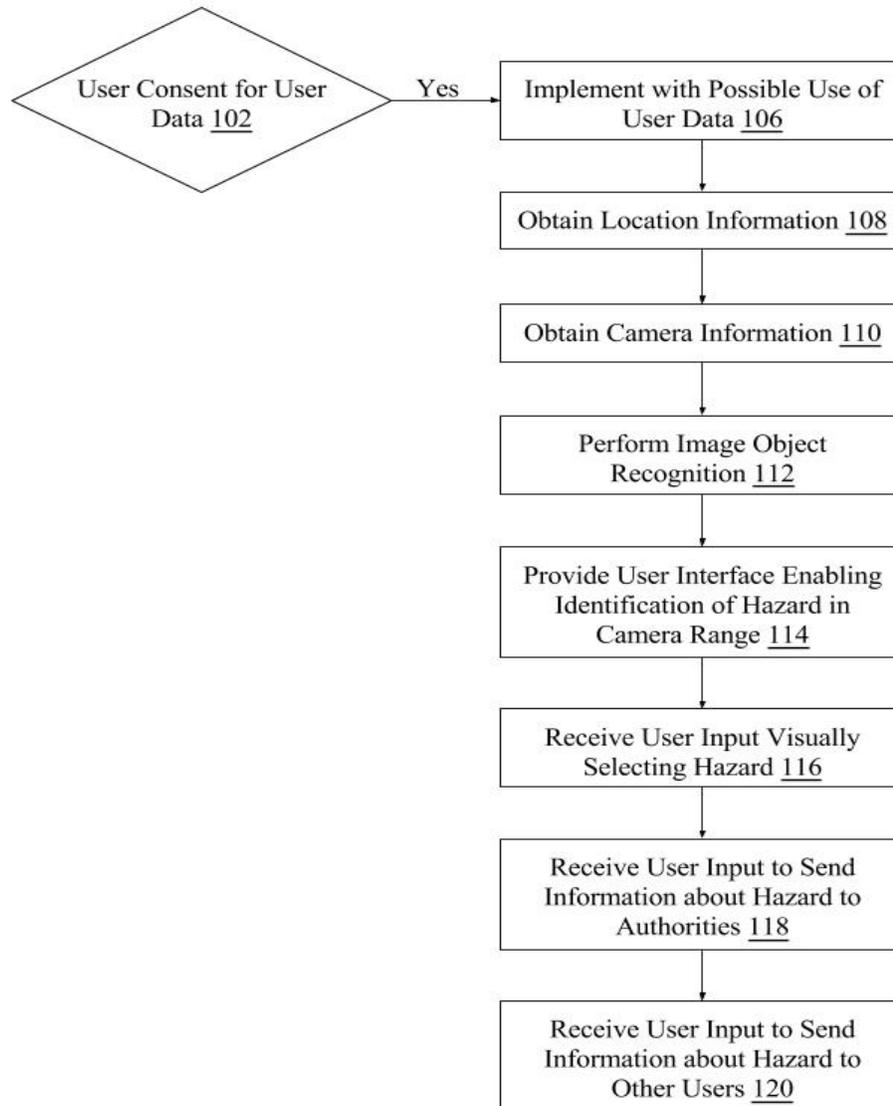
**Fig. 1: Reporting road incidents using in-vehicle camera**
