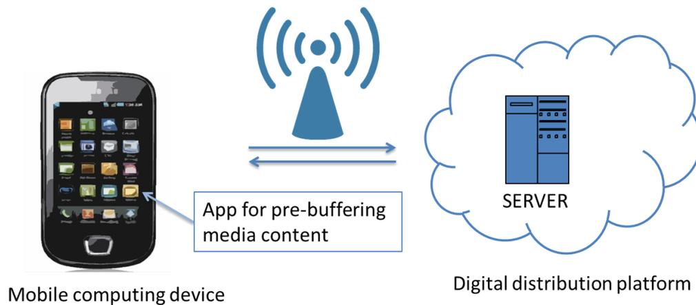
FIG. 1: A system for aggressively pre-buffering media content on a device.
