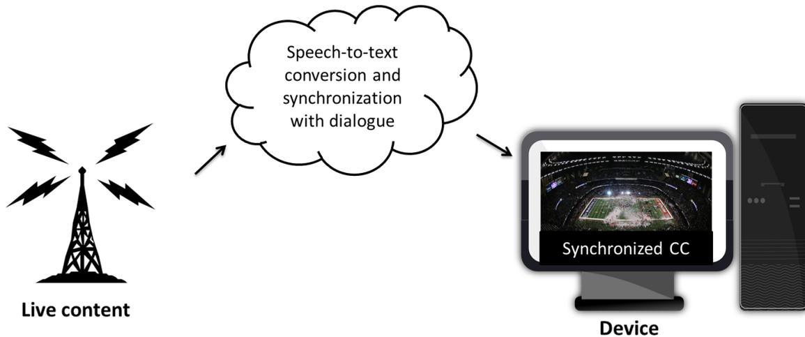
FIG. 1 – A method for providing synchronized CC for live content
