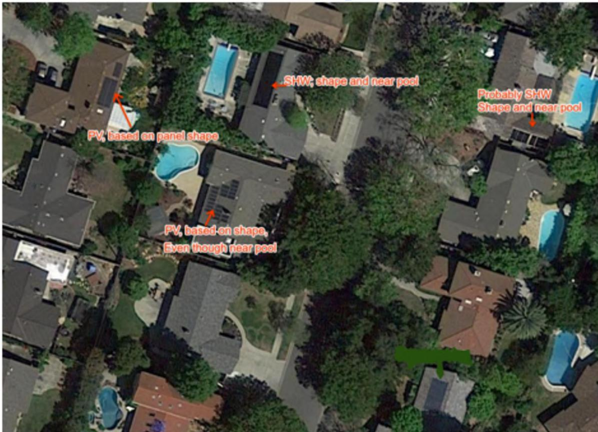
**Fig. 1: Example aerial image used to detect location and parameters of solar arrays.**
