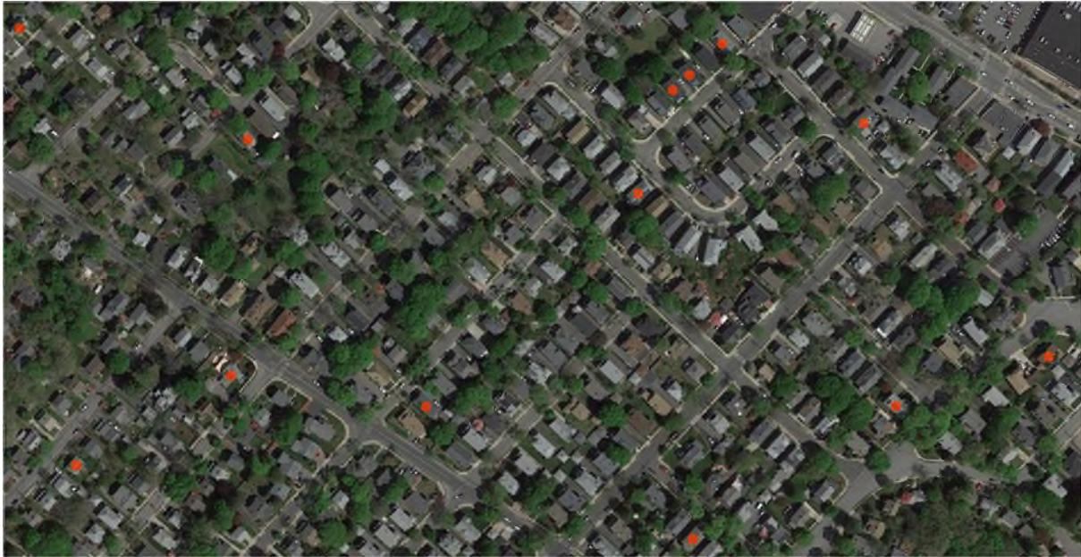
**Fig. 3: An example of detected solar panels overlaid on a map**
