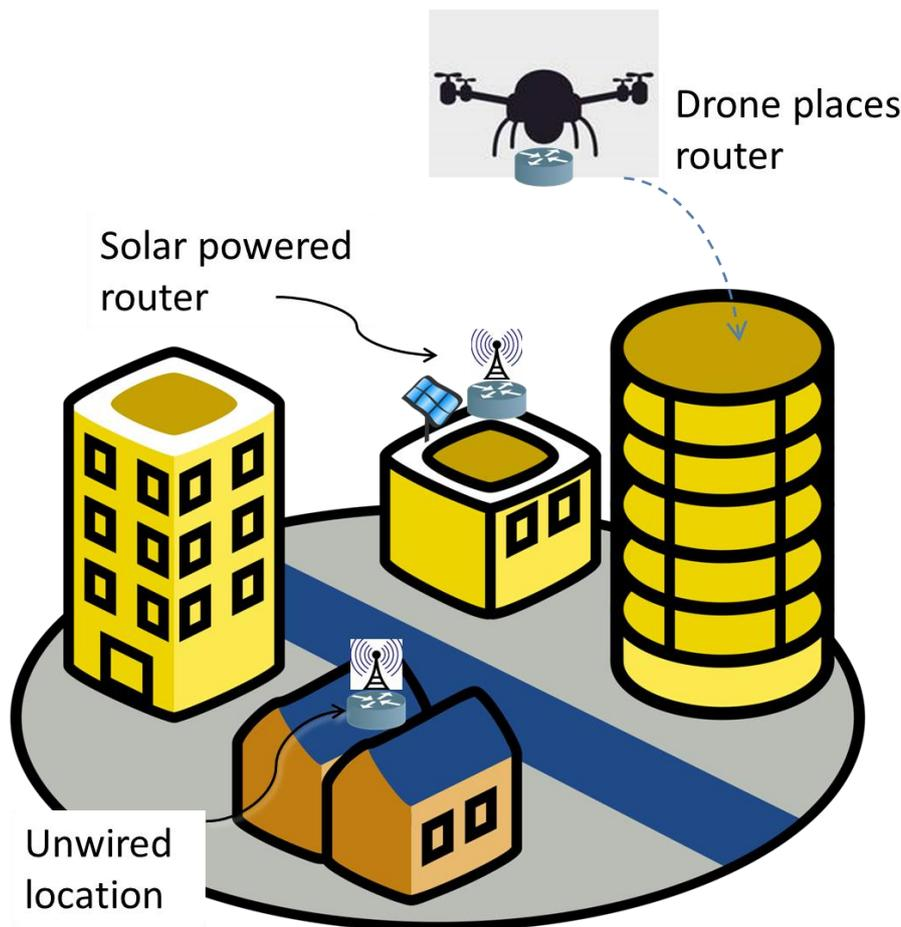
FIG. 1: System for extending internet access via fast deployable portable routers
