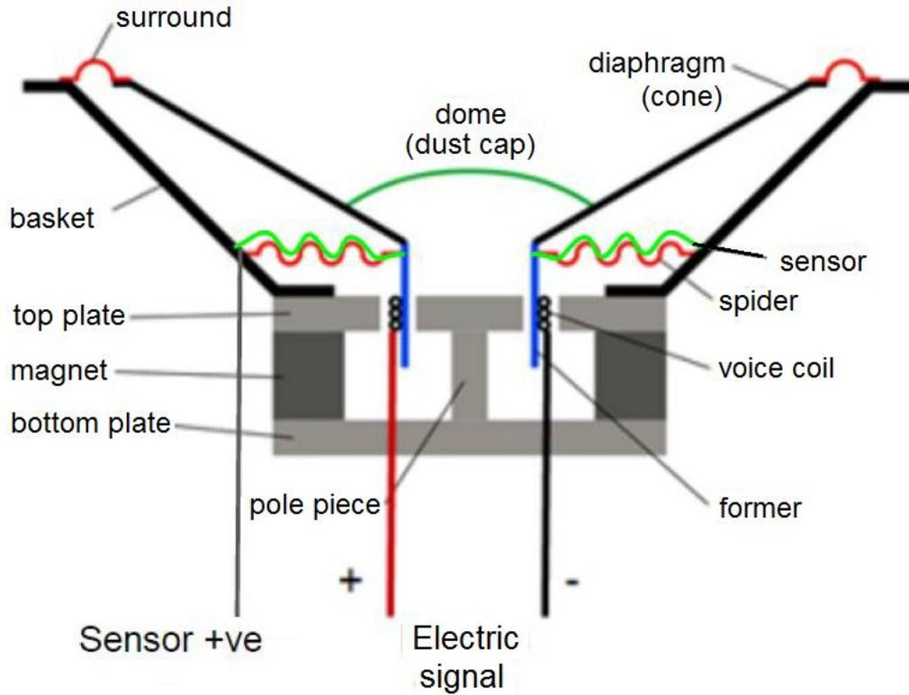
FIG. 1: Device for excursion sensing on the surround of an acoustic transducer
